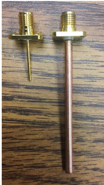
Figure 13. SMA Connector, left, and SMA Connector with copper extension
