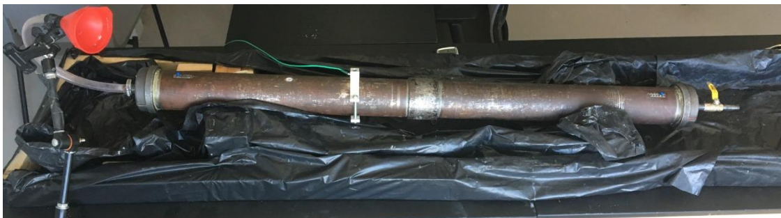
Figure 20. Spill containment setup
