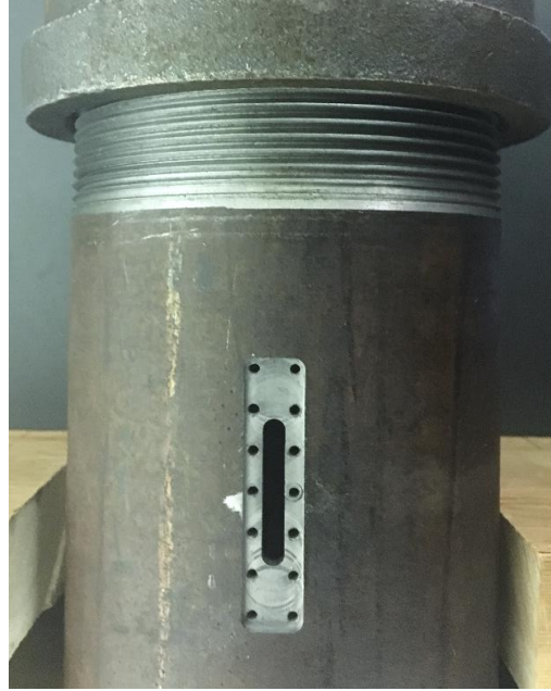
Figure 15. Probe Plate CAD drawing, left, and modified pipe
