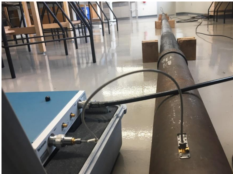
Figure 24. Long section of pipe being measured with the VNA
