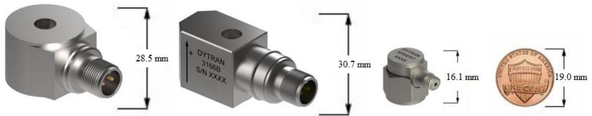
Figure 17: Dytran accelerometers used on shake table and blocks: series 3202 (left), series 3166 (middle), and series 3055 (right) (Dytran, 2019)
