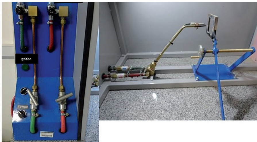
Figure 1. Oxyacetylene torch test equipment scheme.
