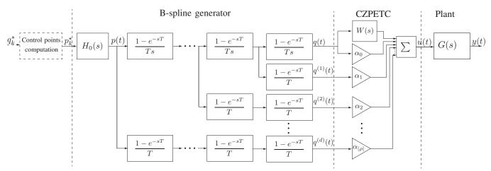
Fig. 2. Block-scheme representation of feedforward control based on B-spline trajectory generator and CZPETC ( $d = |\rho|$ ) for the plant G(s).
