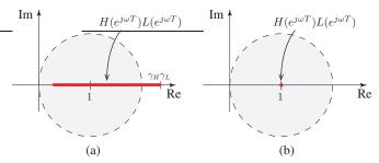
Fig. 8. Stability region for P(z) in the RC scheme of Fig. 4: typical Nyquist plots of  $P(e^{j\omega T})$  obtained with non-minimum phase plant (a) and of a minimum phase plant (b) with CZPETC. In both cases the gain  $K_p$  is not considered, i.e.  $K_p = 1$ .
