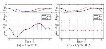
Fig. 16. Output signal y(t) and tracking error obtained with the CZPETC-RC based on  $G_{5p2z}(s)$  during the iteration #0 (a) and the iteration #15 (b).
