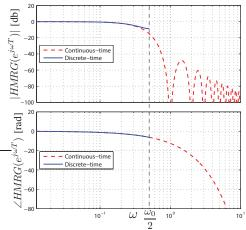
Fig. 7. Frequency response of a discrete-time system HMRG(z) obtained by sampling (with period T) the continuous-time system  $H_0(s)M^d(s)R_{\text{ZPET}}(s)G(s)$  with d = 3 and G(s) with an unstable zero.
