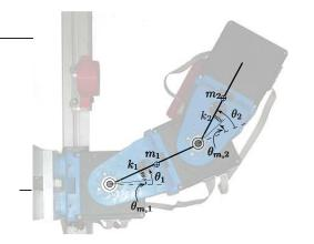
Fig. 9. Two-link robotic arm with elastic joints based on QBMove - Maker Pro VSAs.
