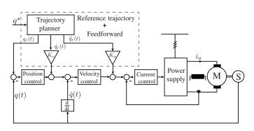
Fig. 1. Standard cascade control structure with feedforward for electrical motor drives [17] .
