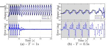
Fig. 13. Output signal y(t) and tracking error of the RC scheme without CZPETC for different values of the knot span T.
