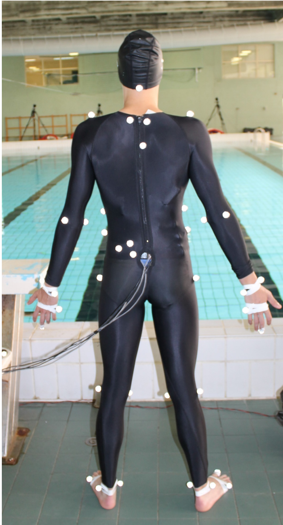
Figure 5-5. Qualisys marker locations – rear view. The hole in the swimsuit to allow the EMG cables to exit is also visible.
