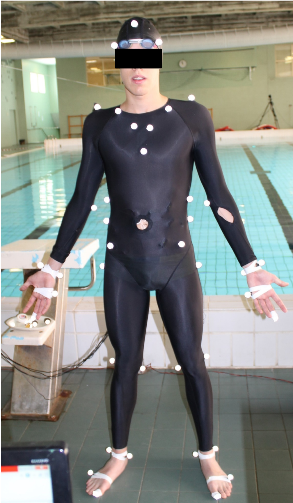
Figure 5-4. Qualisys marker locations – front view.
