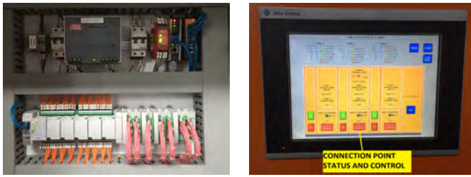
Fig. 9. CP programmable logic controller and human-machine interface.
