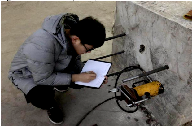
Fig. 6. Pullout test using concrete block.
