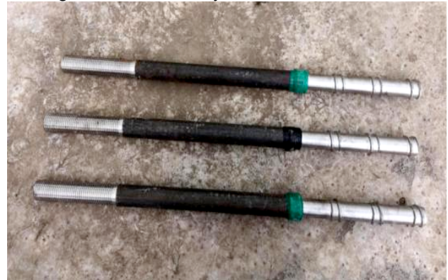
Fig. 8. C1 bolt used for field test
