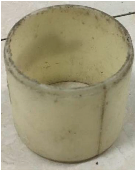
FIGURE 2: \text{Ø}50 \times 50 plastic mould.
