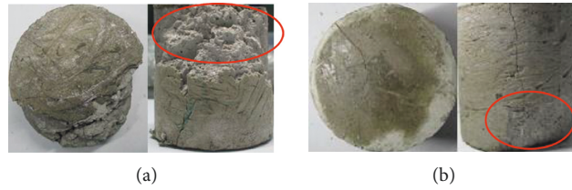
FIGURE 7: Typical failure modes of foam concrete under impact loading. (a) S-4-5. (b) S-0-3.
