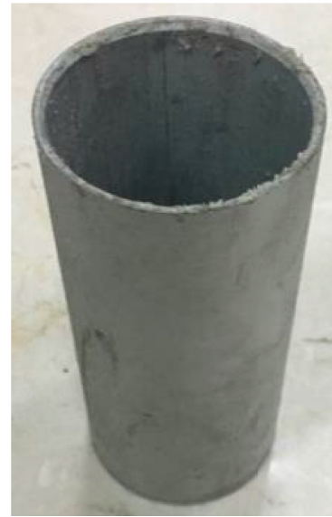
FIGURE 3: \text{Ø}50 \times 100 aluminium mould.
