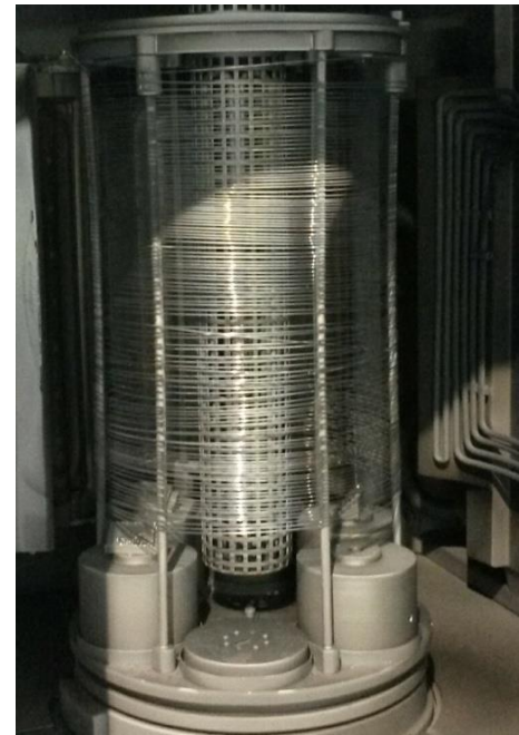
Figure 3: Device for holding the welding wire in the system [7]
