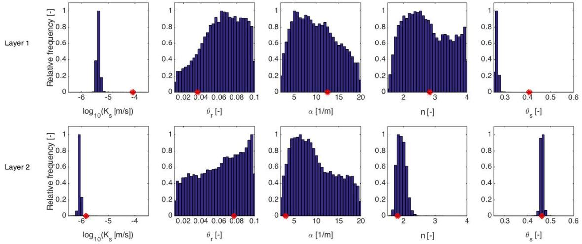
Figure 10: Marginal posterior histograms for the VGM parameters in each soil layer, obtained through MCMC sampling using an  $L_2$ -norm-based likelihood measure for the residuals with no model-error correction (see text for details). The red dots indicate the true parameter values. The limits of the horizontal axis on each plot represent the prior uniform parameter bounds.
