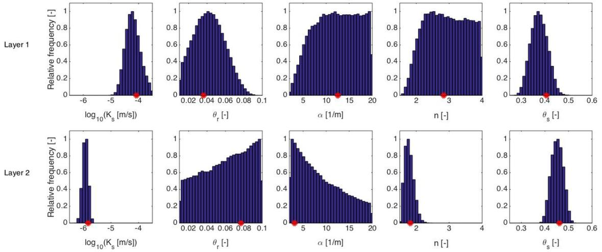
Figure 12: Marginal posterior histograms for the VGM parameters in each soil layer, obtained through MCMC sampling using an  $L_2$ -norm-based likelihood measure for the residuals after correcting for model error (see text for details). The red dots indicate the true parameter values. The limits of the horizontal axis on each plot represent the prior uniform parameter bounds.
