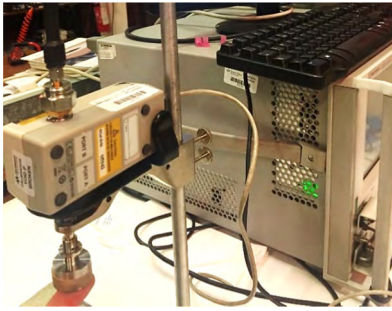
FIGURE 1. The in-house measurement setup based on the open-ended coaxial probe technique, used for the characterization of the dielectric materials.
