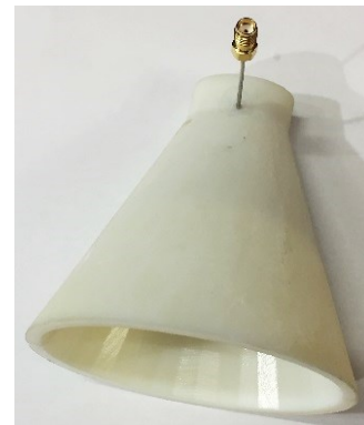
(b). 3D-printed EDRH antenna, as conductive-painted and fed with a semi-rigid SMA connector.
