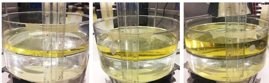
Fig 5. 66: The prepared setup of the developed liquid model, for different oil thicknesses of 10 to 30 mm for the experiment.
