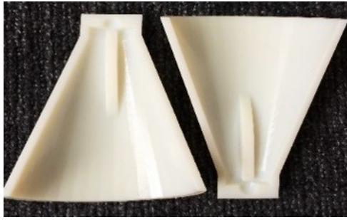
(a). 3D-printed EDRH antenna using the polyethylene material.
