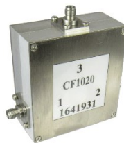
Fig 5. 82: CF1020 Circulator 1-2Ghz VSWR 1.35 S Steel SMA 50Watts.
