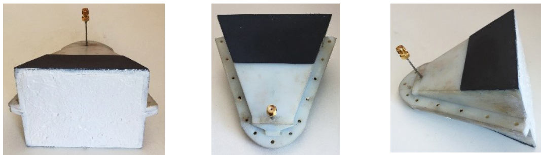
(c): The 3D-printed PDRH antenna filled with the high-dielectric material and the absorbers are glued to lower and upper-extended flares.
