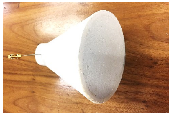
(b). 3D-printed EDRH antenna, as conductive-painted and fed with a semi-rigid SMA connector.
