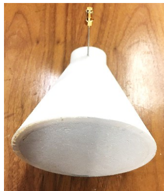
(c). 3D-printed EDRH antenna, filled with the high-dielectric mixture.
