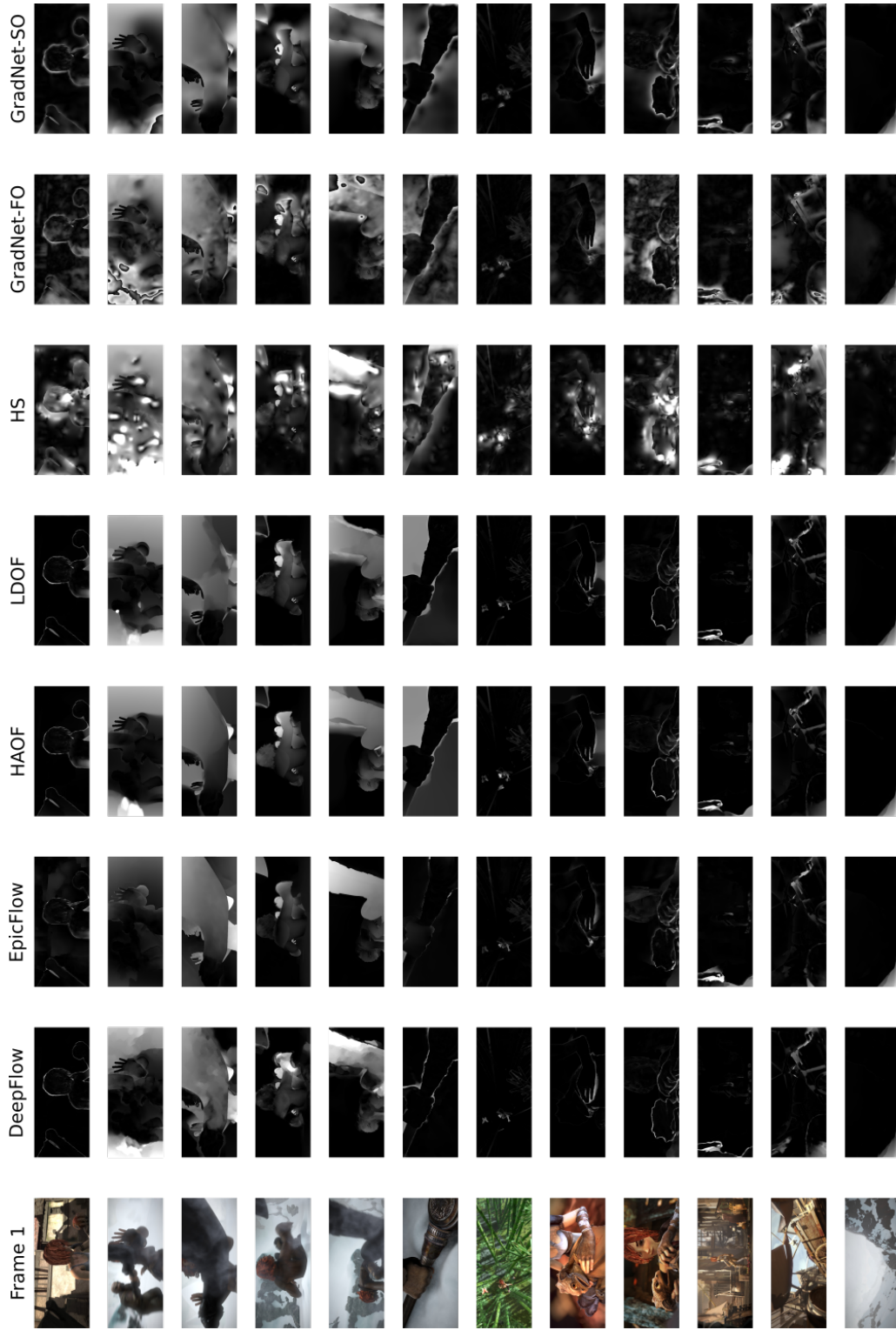
Figure 3.10: The AEE maps calculated for several samples from several methods on MPI-Sintel the final-training split. Each sample is normalized by a factor of \frac{255}{\max(d)} , where d = \sqrt{u_{gt}^2 + v_{gt}^2} . Values more than 255 are rounded to 255.
