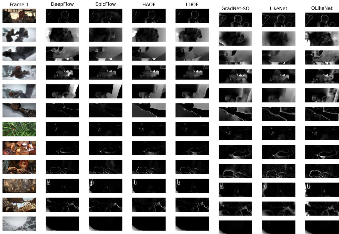
Figure 5.6: Comparison with classic methods. The AEE maps calculated for several samples from several methods on MPI Sintel the final-training split. Each sample is normalized by a factor of \frac{255}{\max(d)} , where d = \sqrt{u_{gt}^2 + v_{gt}^2} . Values more than 255 are rounded to 255.
