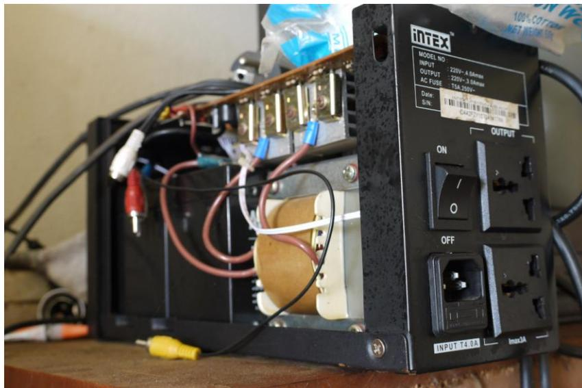
*Figure 3 : Small UPS (Uninterruptible Power Supplies) are frequently used to provide emergency power to a load when the [http://en.wikipedia.org/wiki/Mains\\_electricity](http://en.wikipedia.org/wiki/Mains_electricity) fails. Many of them are damaged by electrical surges like the one on the picture above.*
