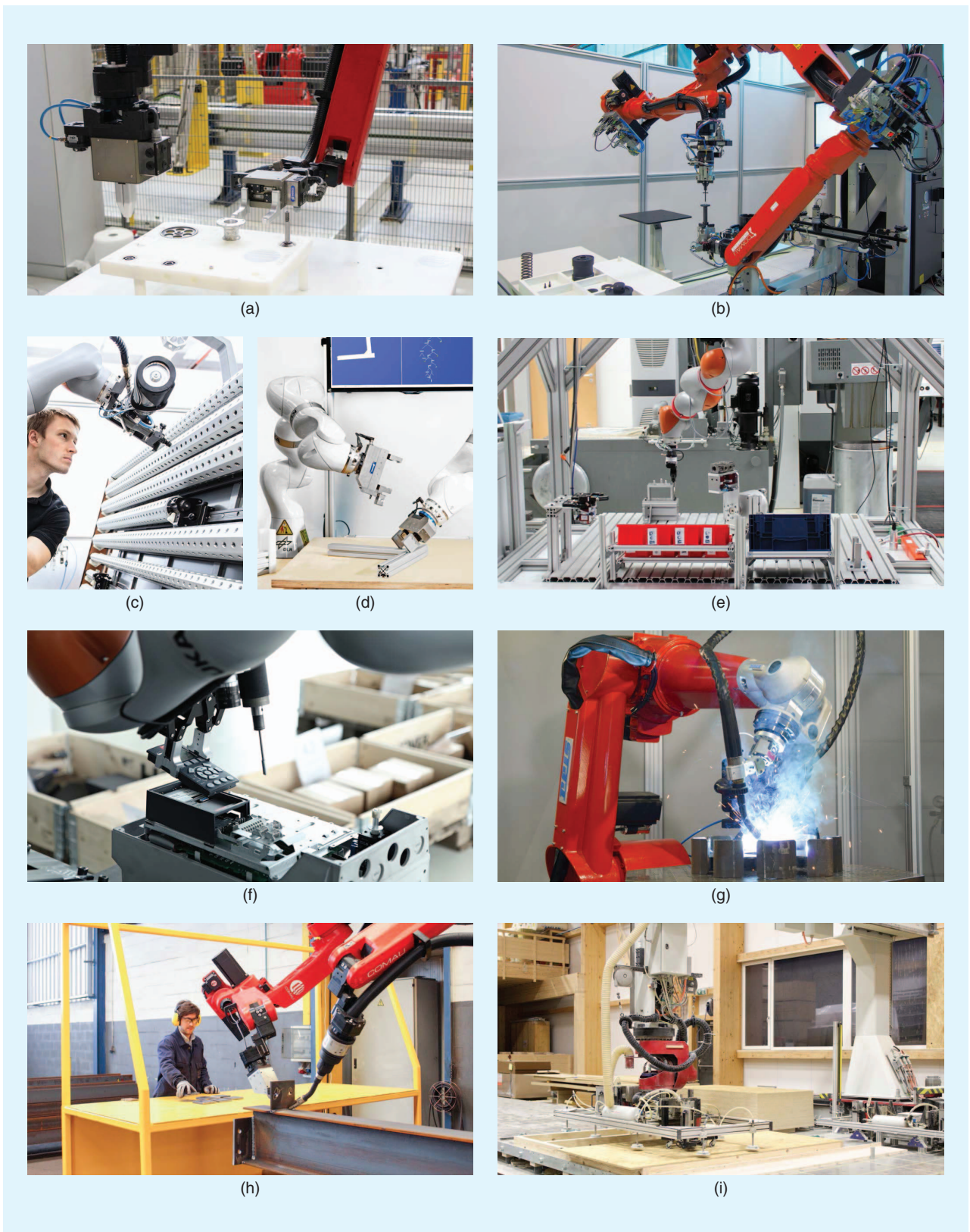
Figure 10. Demonstrators used to evaluate new technologies in the SMERobotics project: the (a) assembly of a gearbox, (b) assembly of a latch valve, (c) riveting for the assembly of custom grippers, (d) assembly of aluminum profiles, (e) assembly of high variants of valves, (f) subassembly of energy converters including tightening screws, (g) smart welding with automatic sensor-based path correction, (h) intuitive teaching of welding tasks, and (i) construction of a wall for a wooden house. [Part (b) courtesy of Tecnalia, Spain; part (c) courtesy of Kuka, Germany; part (d) courtesy of DLR Oberpfaffenhofen, Germany; part (f) courtesy of DTI, Denmark; part (g) courtesy of Fraunhofer IPA, Germany; and part (h) courtesy of INESC-TEC, Portugal.]
