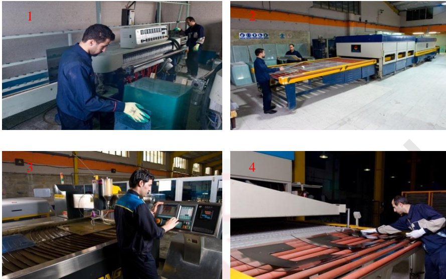
Figure 1.2 Functional shops in glass cut company (Bordering, Sekuritting, Punching and Bending) (Arian Shisheh Company. Retrived at 25.05.2013 from www.arianshisheh.com .)
