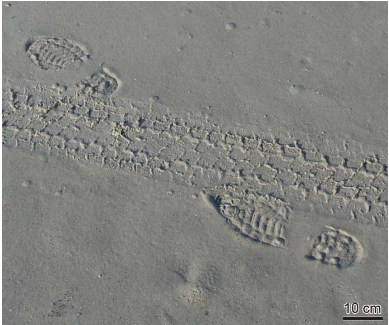
Figure 5. Shoe and tire impression on wet sand demonstrating high-bearing capacity of partially saturated sand affected by capillary cohesion.
