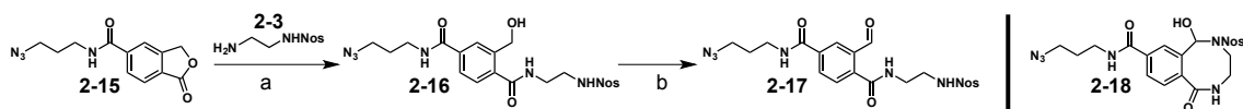
Figure 51. Aldehyde synthesis from lactone 2-15 . Reaction conditions: a) K_2CO_3 , THF, 65°C, 23 h, 62% . b) DMP or IBX, (additives), THF, RT, 15 min, 0% .
