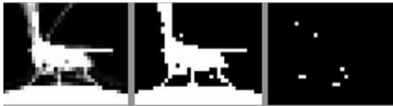
Figure 6.7: Pixel subtraction for movement detection 4 . The difference of images between consecutive frames provides a proxy for movement.
