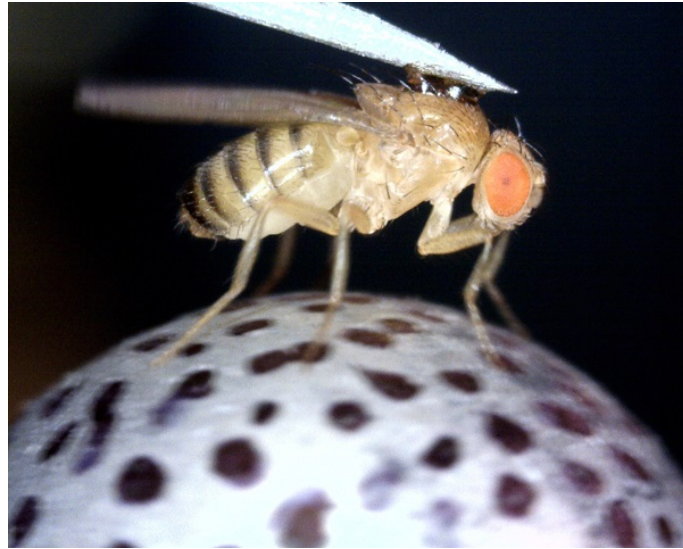
Figure 1.13: Fly on the ball set-up 14 . Here the fruit-fly is allowed to walk on the ball, while the motion of the ball can be used to track the movement of the fly including its walking speed, turning direction etc.
