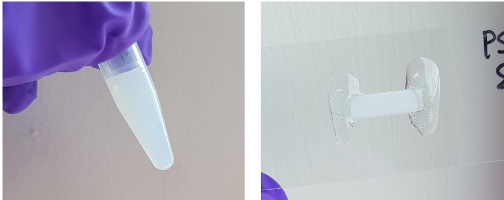
Figure 4.18: Images of 80 nm polystyrene colloids well dispersed in water (left) and quenched into an arrested colloidal gel (right). Blue colour is observed when dispersed but not when gelled.
