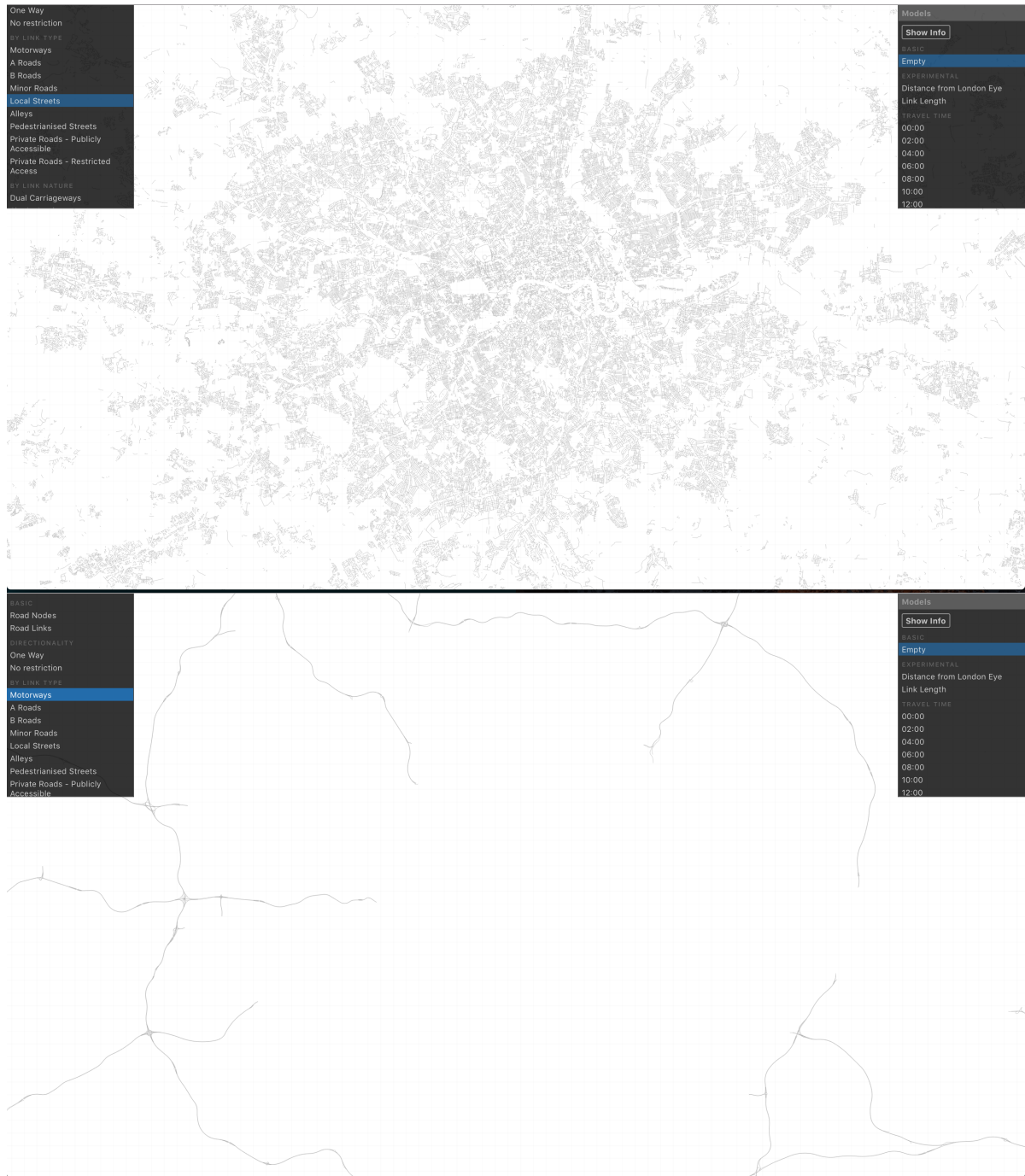
Fig. 4.9 Fundamental components of road graph, aggregated by edge nature. Top - local streets, bottom - Motorways
