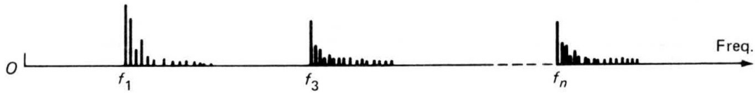
Figure 3-6. Qualitative plot of the overtone spectrum of AT-cut quartz sampled at different harmonic modes. Reprinted from [88].
