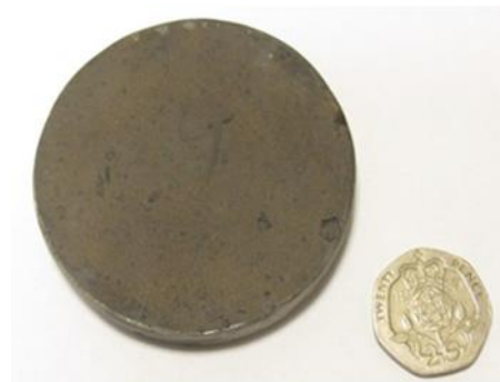
Figure 1. 50 mm diameter MgB 2 hot pressed bulk superconductor.
