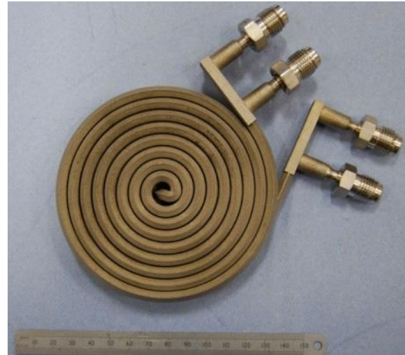
Figure 7. Additively Manufactured prototype spiral heat exchanger.
