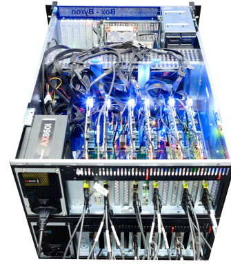
Fig. 10. Our current FPGA cluster comprising two POETS boxes (12 worker FPGAs in total, in a 3 \times 4 arrangement), each in a standard 4U rack-mountable case. Refer to Figure 1 for further details about POETS boxes.
