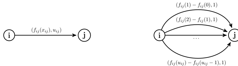
Figure 3.5: Illustrating the transformation of a MCCNFP to a MCNFP on an expanded network. For every arc (i, j) \in A with capacity u_{ij} , there are u_{ij} arcs in the expanded network.
