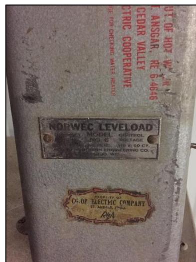
Figures 4.1 and 4.2: Time Clock (Left) and Powerline Carrier Receiver (Right) from an Iowan Electric Cooperative. Early permutations of load management were relatively plug-and-play, such as time clocks, which with a simple turn of the hand, allowed for customized control of on-farm electricity demand. Powerline carrier receivers, requiring more advanced communication over power lines, were more advanced, requiring communication networks to be set up. Source: Dairyland Power Cooperative personal communication.
