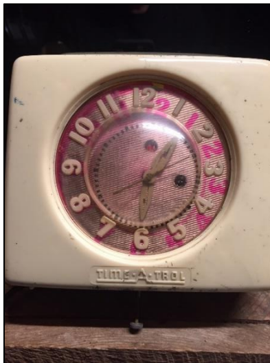
Figures 4.1 and 4.2: Time Clock (Left) and Powerline Carrier Receiver (Right) from an Iowan Electric Cooperative. Early permutations of load management were relatively plug-and-play, such as time clocks, which with a simple turn of the hand, allowed for customized control of on-farm electricity demand. Powerline carrier receivers, requiring more advanced communication over power lines, were more advanced, requiring communication networks to be set up. Source: Dairyland Power Cooperative personal communication.
