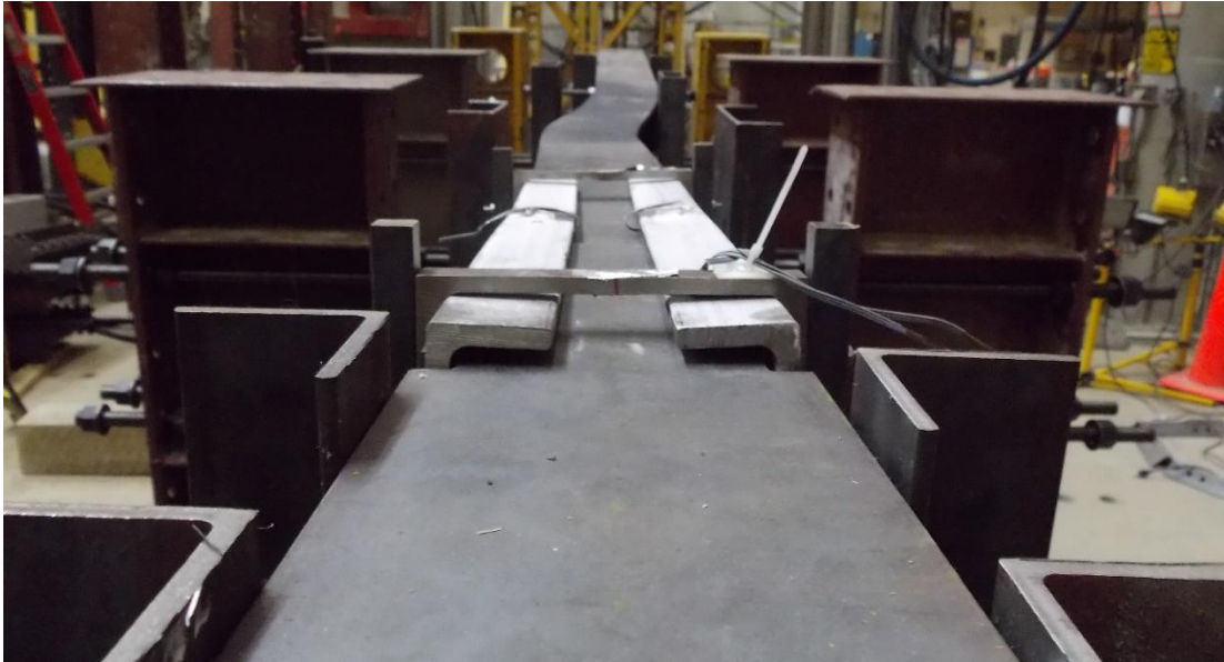
Figure 5.5.12: Deformed beam shape after bracing was loosened
