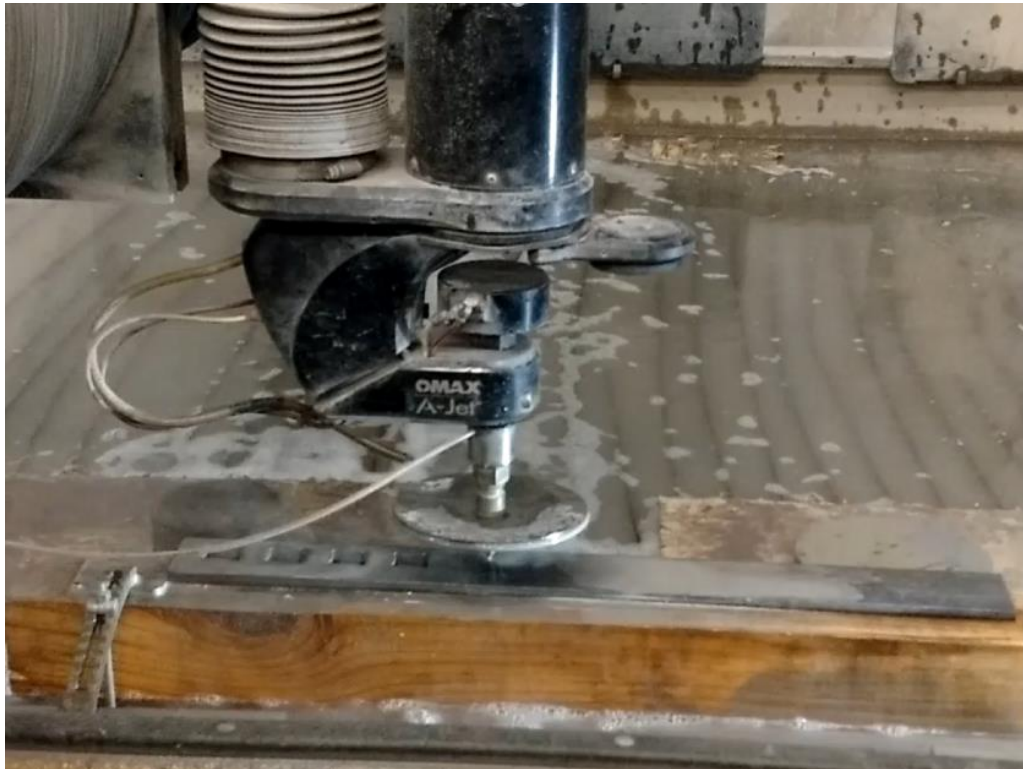
Figure 4.2: Water jet cutting
