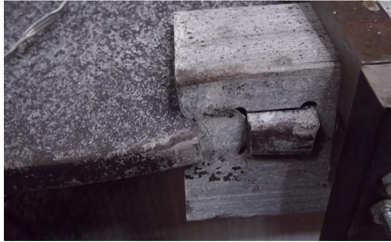
Figure 6.8.1: Local plasticity in Test 3
