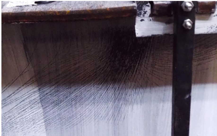
Figure 5.3.11: Web strains in whitewash
