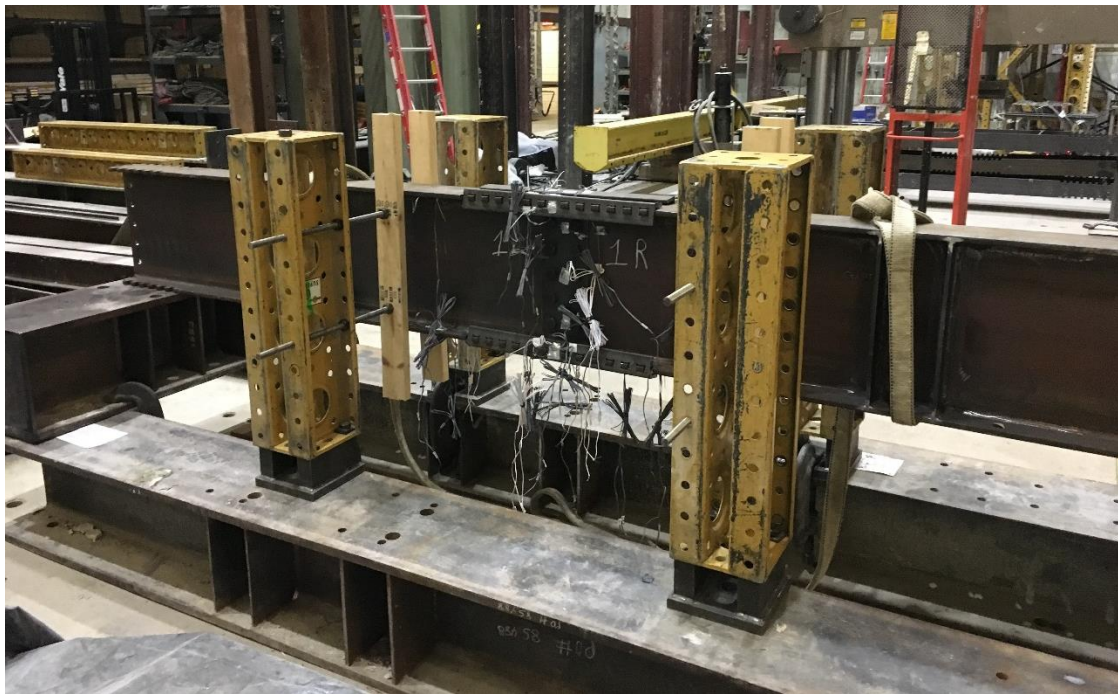
Figure 4.22: Test beam with temporary wood bracing
