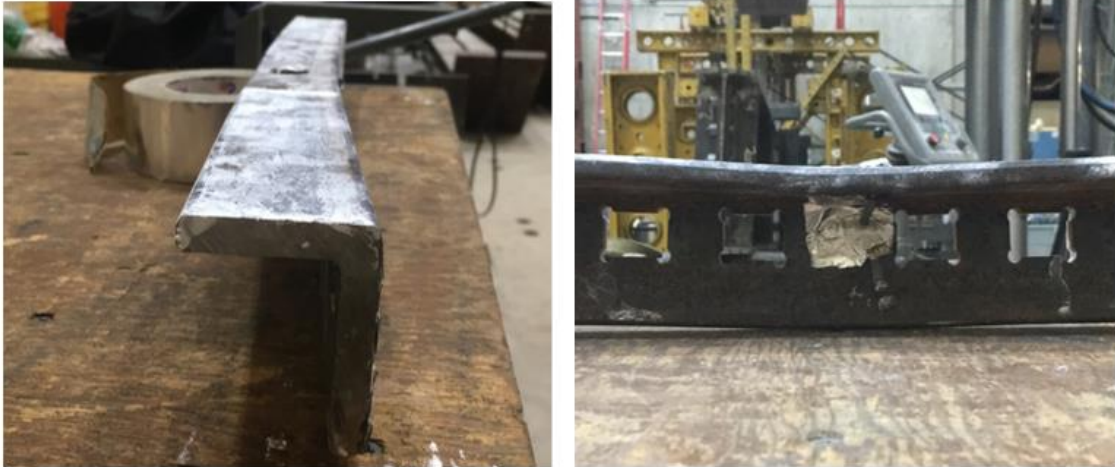
Figure 5.1.11: Test 1 compression angle buckling
