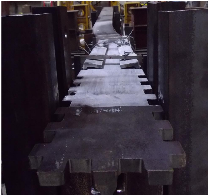
Figure 5.4.13: Test 3 beam deformed shape
