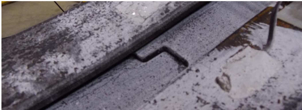
Figure 5.3.2: Test 2 uneven top flanges after testing
