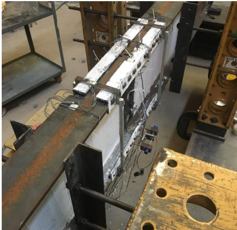
Figure 4.24: Bracing with steel angles in place
