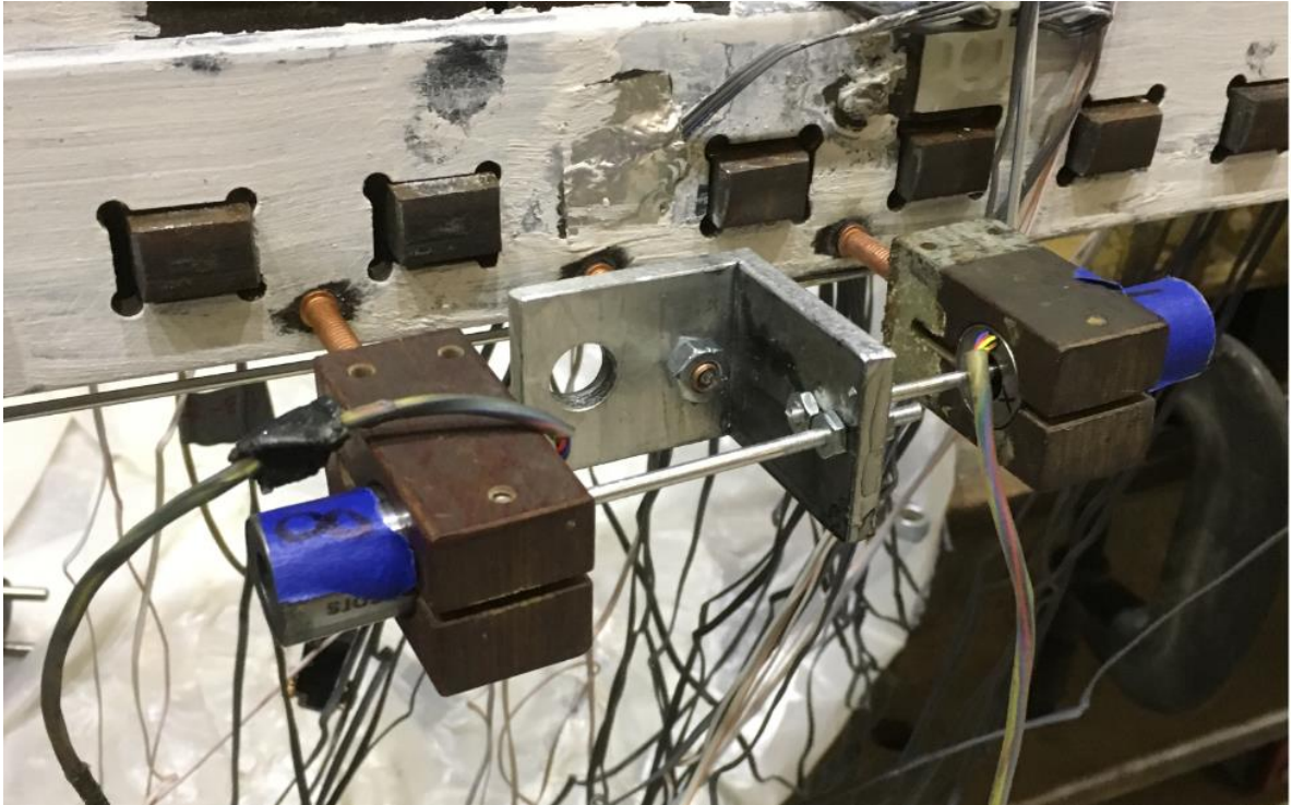
Figure 4.25: LVDT attachment to tension angle
