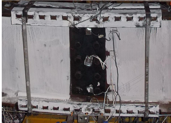
a) Test 1 angle deformation with no shear
