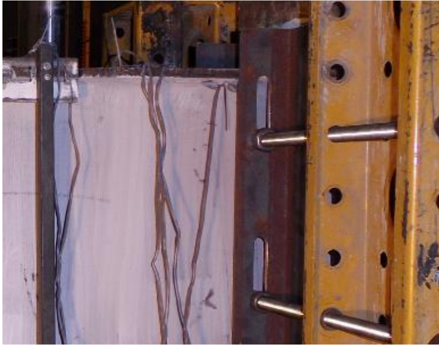
Figure 5.2.1: Bracing slotted holes
