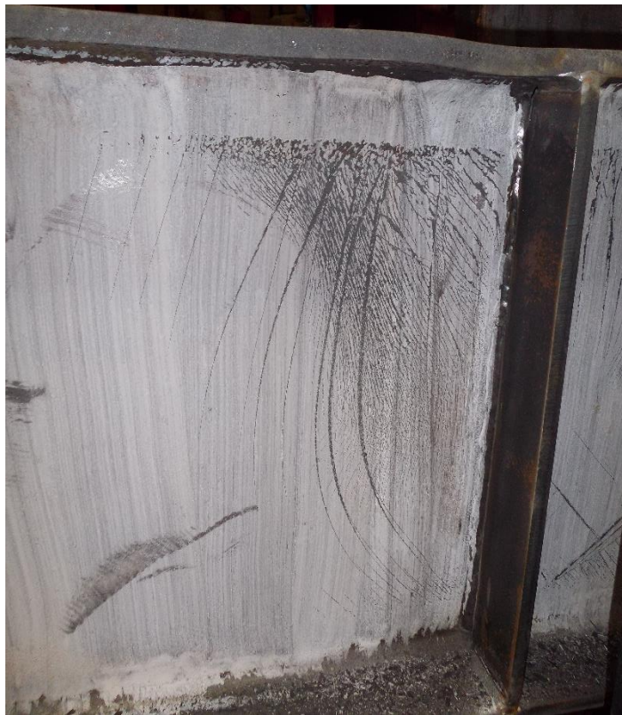
Figure 5.5.13: Shear yielding observed outside the constant moment region
