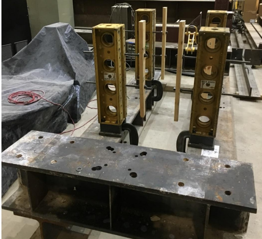
Figure 4.20: Bracing with temporary wood braces
