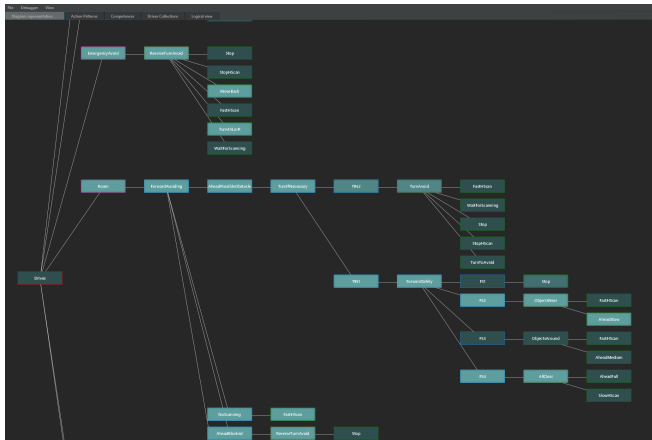
Fig. 3. The ABOD3 Graphical Transparency Tool displaying a POSH plan in debugging mode. The highlighted elements are the ones recently called by the planner. The intensity of the glow indicates the number of recent calls. ABOD3 (used as an IDE for the entire hierarchical cycle) show everything ABOD3-AR uses parts only (2 levels only).
