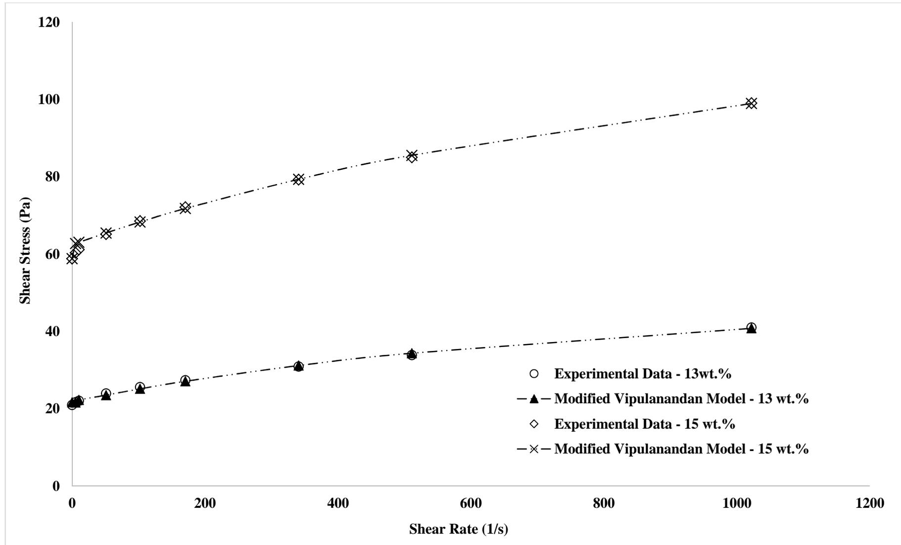
**Figure 4:** Fitted modified Vipulanandan model to rheological data for drilling mud containing 13, 15 wt.% bentonite clay and 0.2 vol.% silica nanoparticles at 25°C
