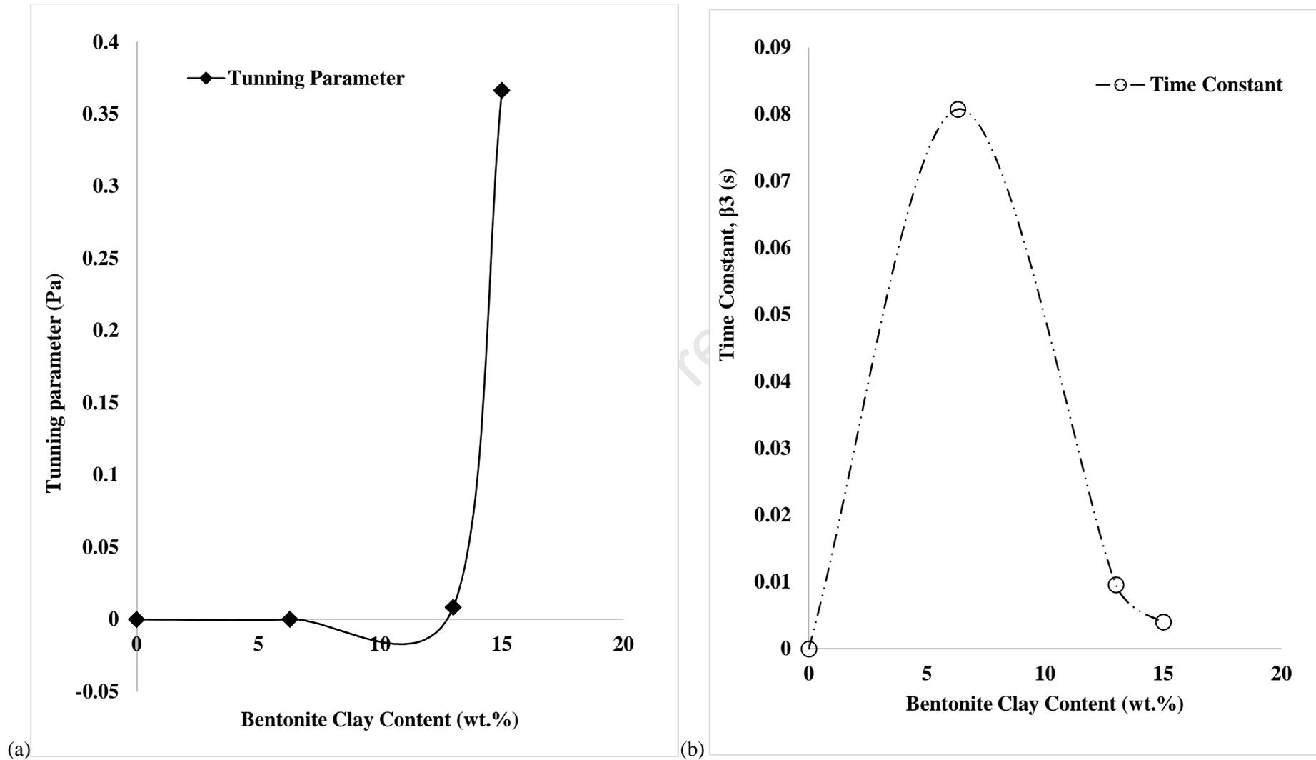
**Figure 5:** Effect of bentonite content on (a) the tuning parameter,  $\beta_0$  and (b) the time constant,  $\beta_3$  for a drilling mud containing 0.2 vol.% silica nanoparticles at 25°C.
