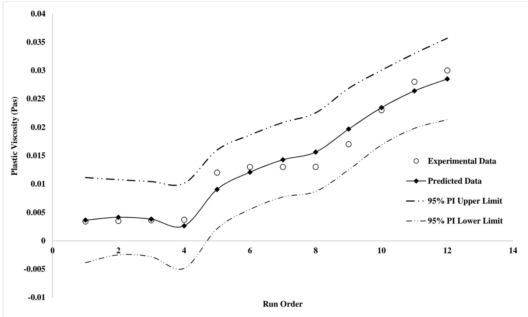
**Figure 8:** The 95% prediction interval (PI) for the statistical model obtained for plastic viscosity in (21) using the experimental design matrix of Table 4.
