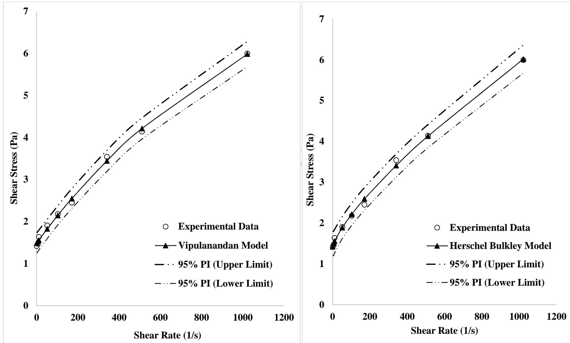
**Figure 3:** The prediction for Vipulanandan and Herschel Bulkley models at 95% prediction interval (PI) using viscometric data obtained for 6.3 wt.% bentonite mud at a temperature of 25°C
