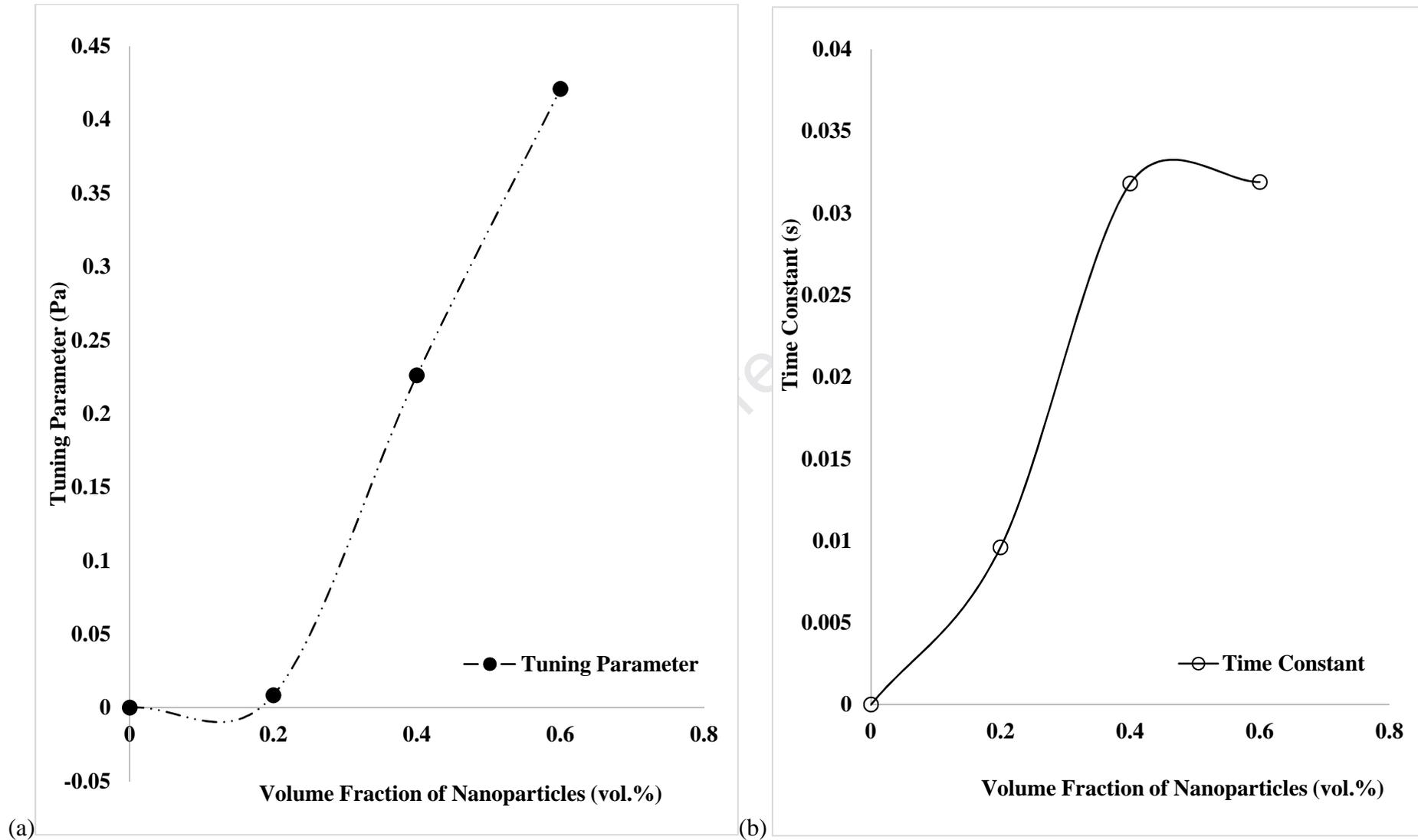
**Figure 6:** Effect of volume fraction of nanoparticles on (a) the tuning parameter,  $\beta_0$  and (b) the time constant,  $\beta_3$  for a drilling mud containing 13 wt.% bentonite clay at 25°C.
