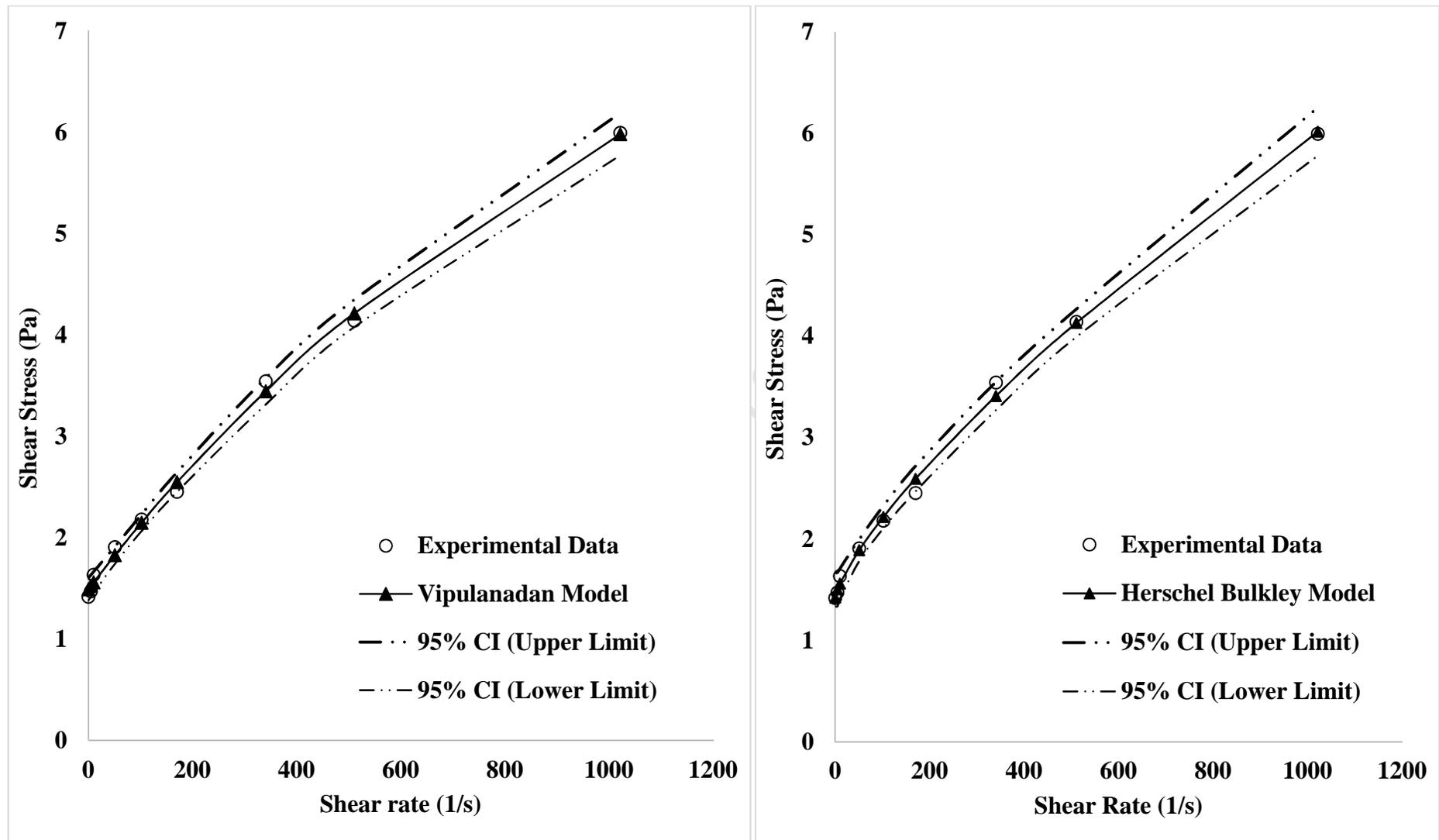
**Figure 2:** The prediction for Vipulanandan and Herschel Bulkley models at 95% confidence interval (CI) using viscometric data obtained for 6 wt.% bentonite mud at a temperature of 25°C
