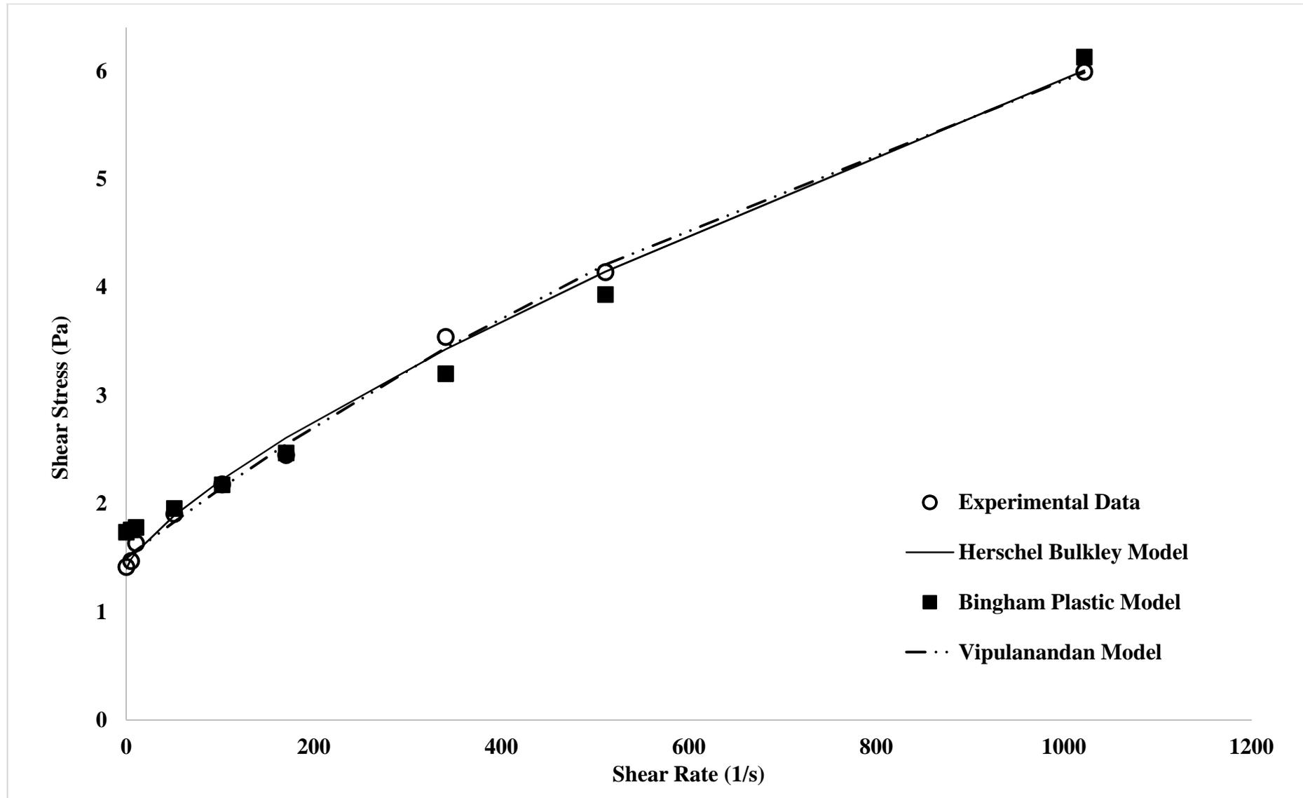
**Figure 1:** Rheological models applied to viscometric data obtained for 6.3wt.% bentonite mud at 25°C
