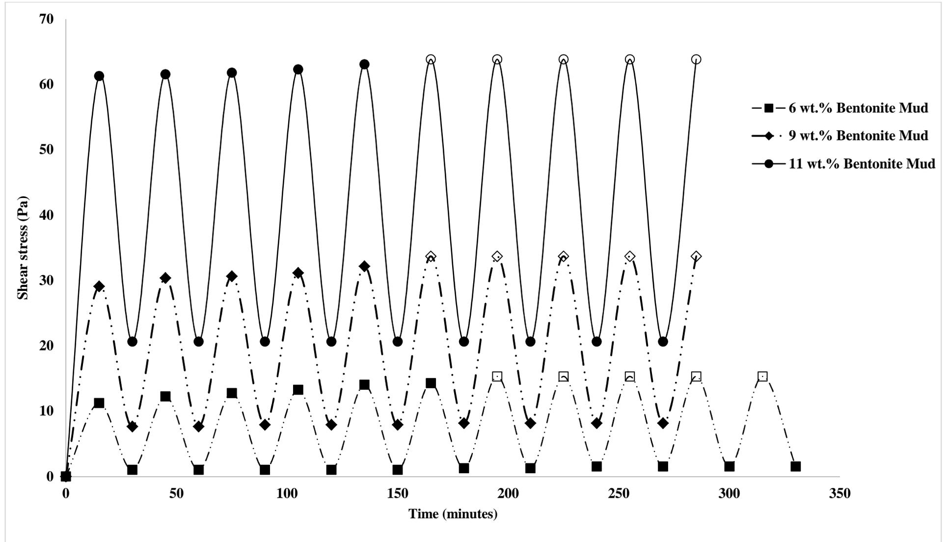
**Figure 9:** Experimental validation results for shear stress limit prediction for 6, 9 and 11 wt.% bentonite mud at shear rate of  $1022 \text{ s}^{-1}$  and temperature of  $25 \text{ }^{\circ}\text{C}$ . The open marker (no fill) corresponds to the constant shear stress values, which approximates the shear stress limit predicted by equation (24).
