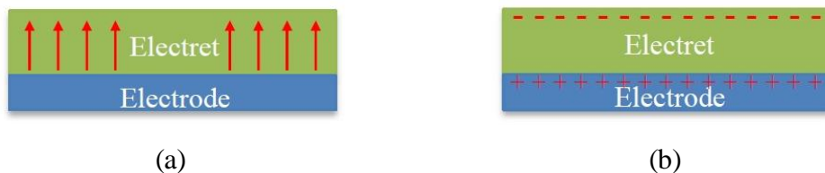
Figure 1.13 Two different types of electrets for electret based electrostatic harvesters (a) dipole orientation and (b) charge injection.
