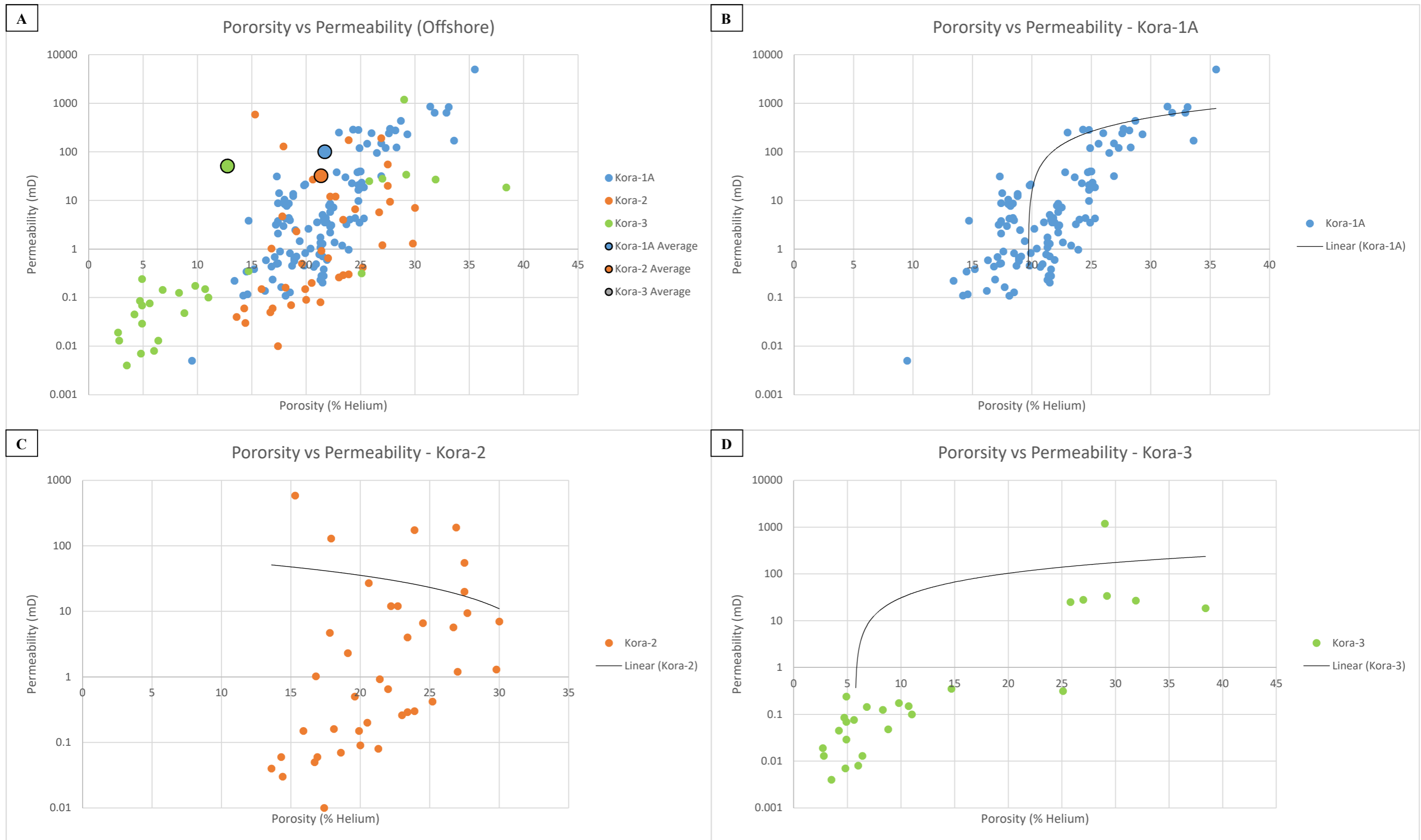
Figure 3.17: A collection of graphs where porosity is plotted against permeability for each well and for all the wells plotted together. A) A graph of helium porosity plotted against permeability for Kora-1A, Kora-2 and Kora-3 wells. B) A graph of helium porosity plotted against permeability for the Kora-1A well. C) A graph of helium porosity plotted against permeability for the Kora-2 well. D) A graph of helium porosity plotted against permeability for the Kora-3 well. All of these graphs have a linear trend line to supplement them, and this provides a an additional feature by which the difference between the average values at each end of the graph can be judged. It is also key to note that the graphs are logarithmic.
