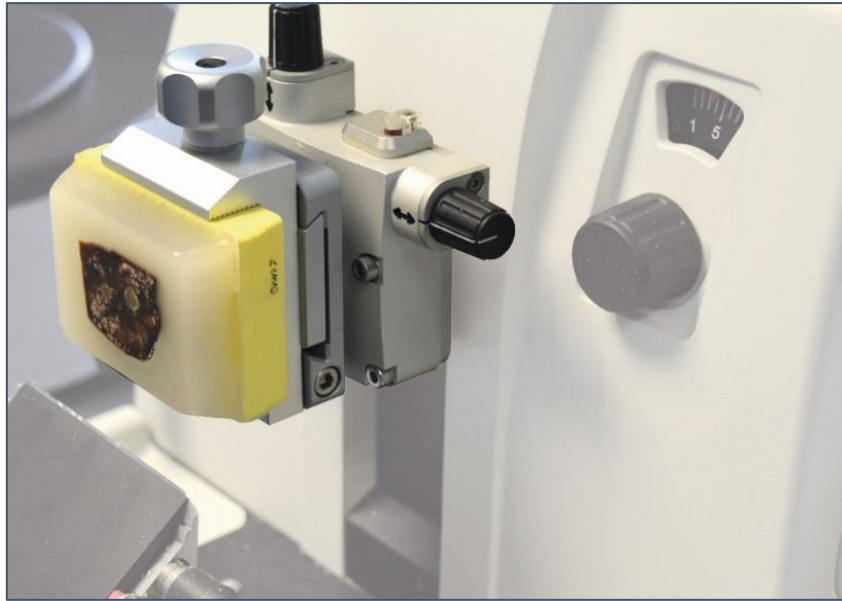
Figure 17. Vice clamps with large metal screw for SM cassettes are slower to use than quick release clamps. If blocks need to be recut or recooled, it takes practice to return them to the same position and not waste tissue.
