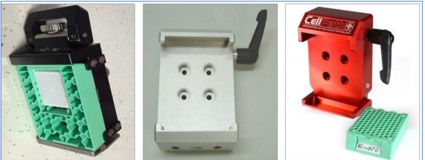
Figure 14. Three styles of SM quick release clamps used for microtomy.
