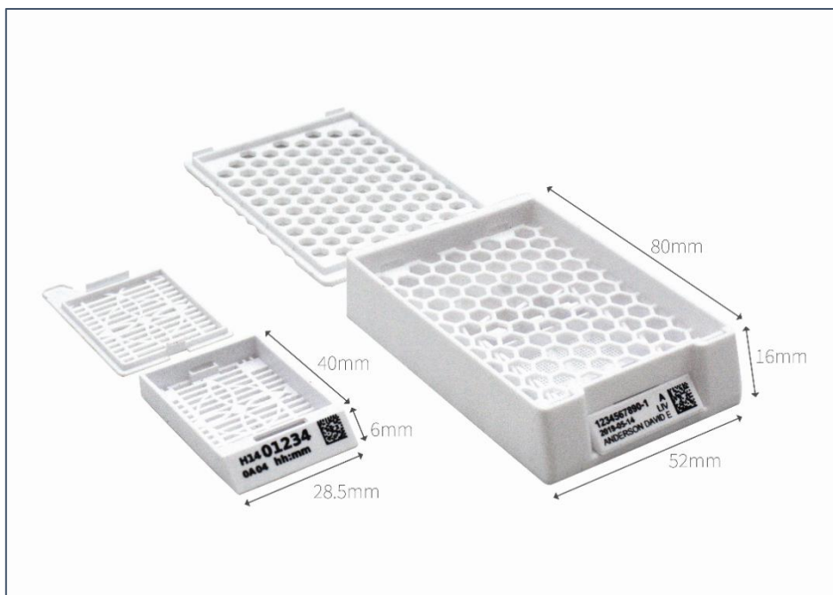
Figure 2. Comparison of a large format processing cassette with one of standard size to show an increased capacity by the larger cassette. Dimensions are shown in mm.
