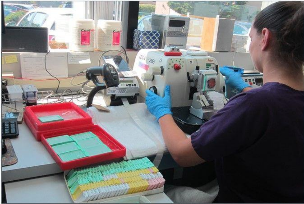
Figure 15. Sectioning large format blocks in the laboratory using a dedicated microtome.
