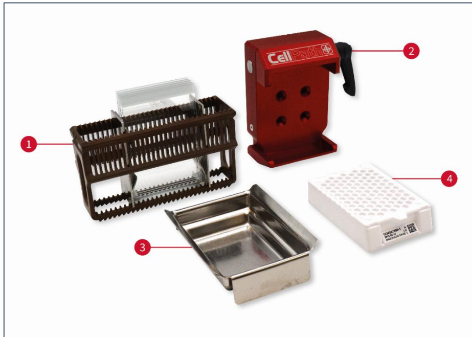
Figure 1. Essentials required for setting up large format include [1] slides and staining rack with adapters, [2] cassette clamp, [3] embedding molds and [4] processing cassettes.
