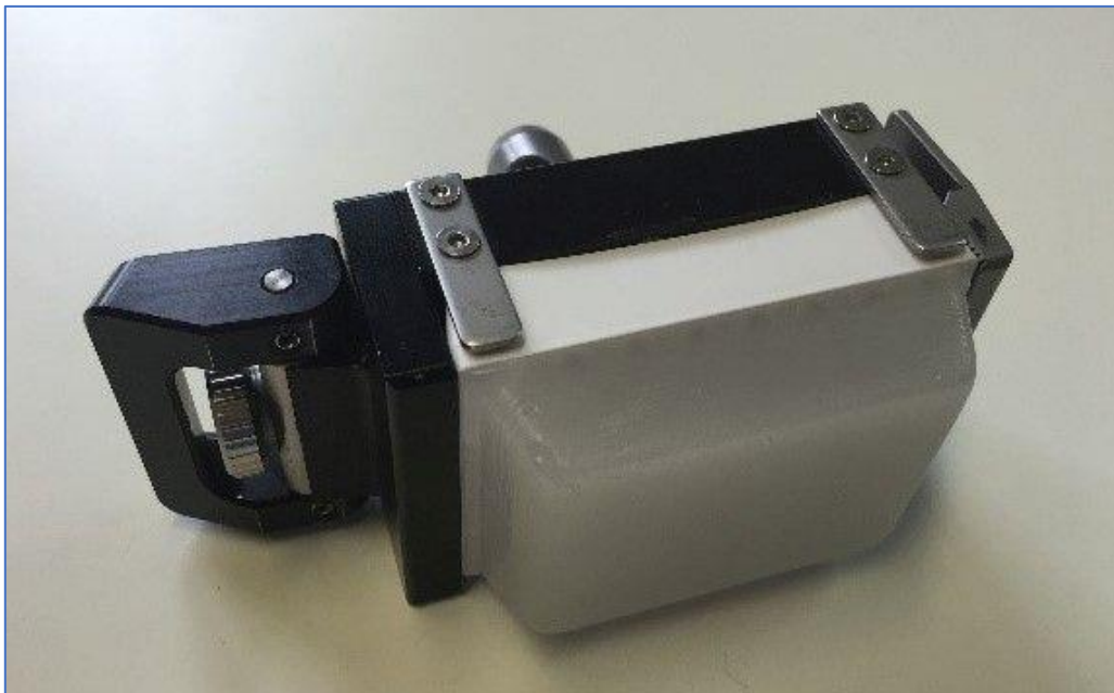
Figure 16 – Longer replacement support plates for the Microm adjustable universal macro cassette clamp. Note the silver arms shown on top of clamp holding the SM cassette with paraffin block. These arms on the longer plate provide improved stability for SM blocks during sectioning when the clamp is in the horizontal position as shown.
