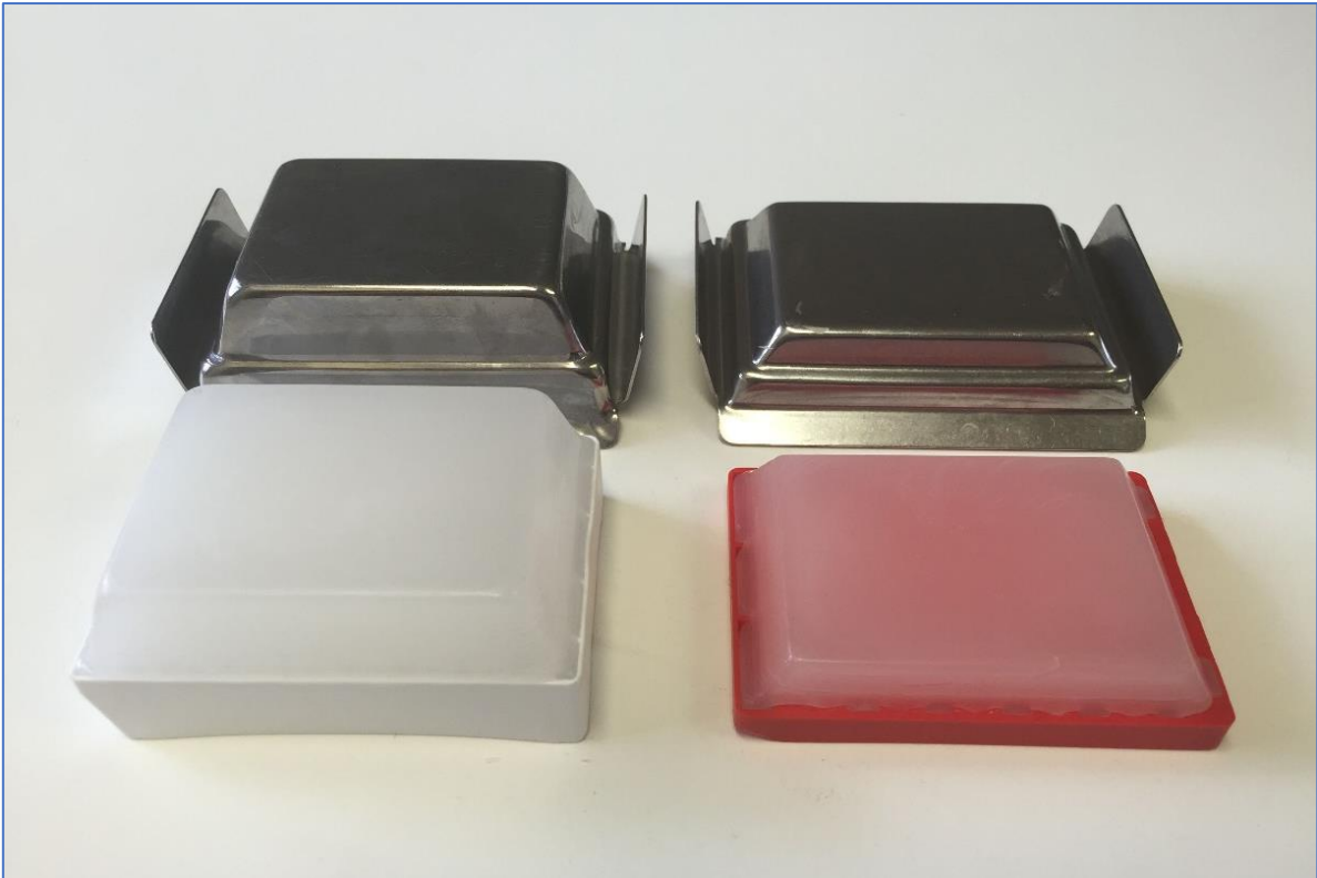
Figure 13. Tissue blocks in deeper metal SM molds take up to an hour for paraffin to harden completely (white). Paraffin blocks for mothership and slim molds (red) will solidify much quicker.
