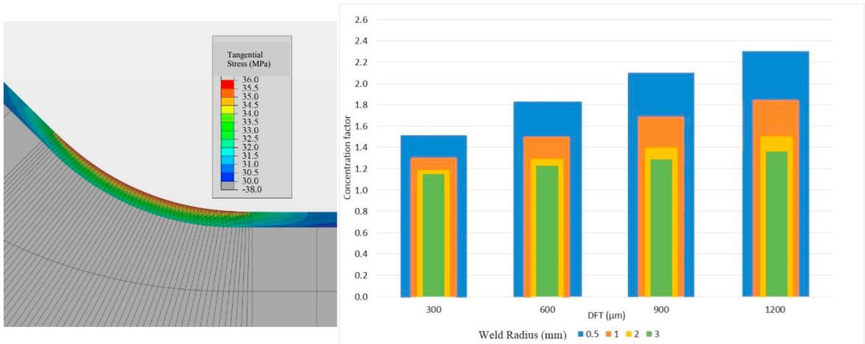
Figure 5: Left - Tangential stress in weld fillet radius at  $-10^{\circ}\text{C}$  after a temperature reduction from  $60^{\circ}\text{C}$ ;
