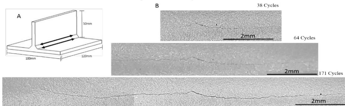
Figure 2: A - Illustration outlining the location and direction of channelling cracks observed;
