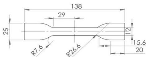
Figure 1: Dimensions (mm) of free film samples
