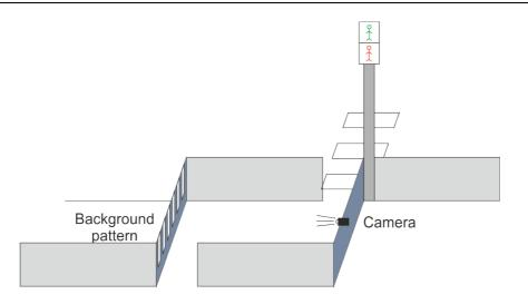
Fig. 6. General scheme of the pedestrian detection system
