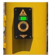
Fig. 1. Button of a traffic light for alerting the system a pedestrian is waiting
