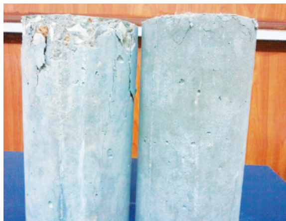
Figure 7. Post crack ductility shown both in cylinder and cube specimens
