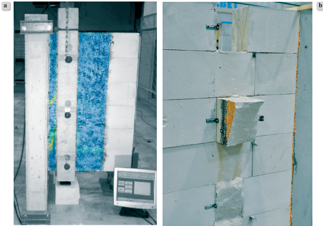
Figure 3. Failure of a P series model a) first cracks in the reference model P_2 b) view of the joint at the moment of failure P_3
