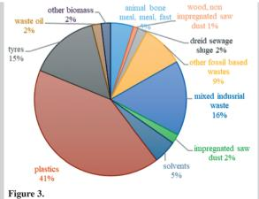
The morphological composition of alternative fuels used in the cement industry, data from 2014 [17]
