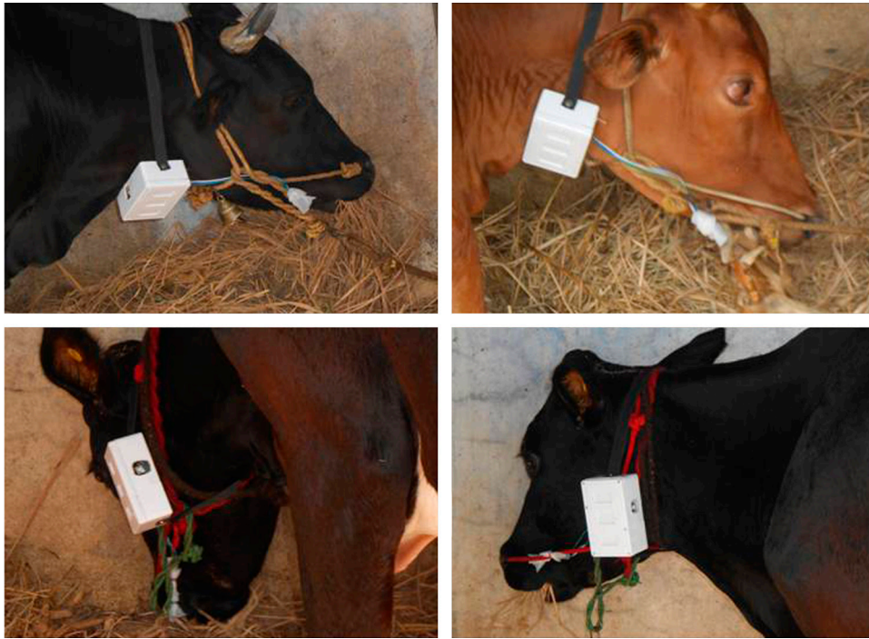
Figure 3: Developed compact device on cattle.
