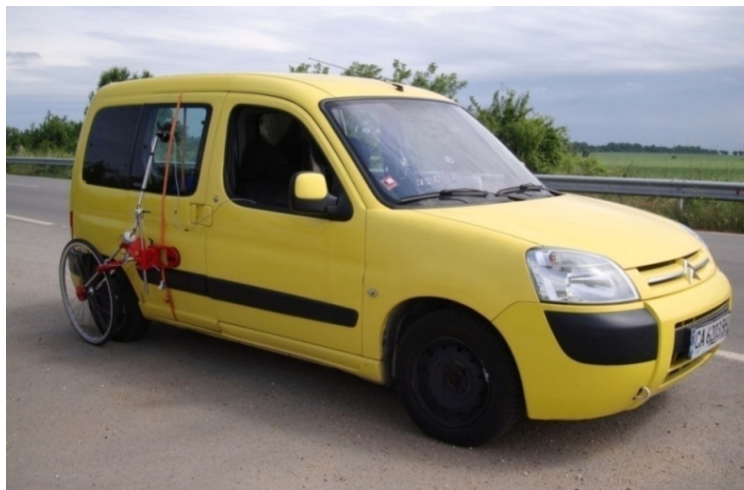
Fig. 5. The tested electric vehicle, equipped with a Peiseler tracking wheel and DB print (in the cab)
