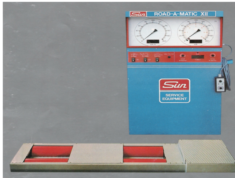
Fig. 4. General view of the laboratory test facility SUN RAM XII
