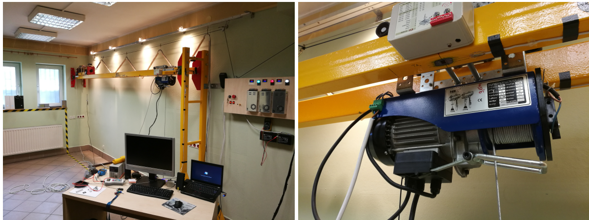
Fig. 1. The test stand: a) supporting structure with the power supply systems, b) vibration exciter PROLIFTOR 250
