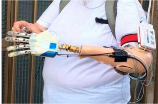
Figure 27: The prosthetic hand containing sensors and electrodes which allow to “feel” in real-time the shape, roughness and consistency of the grasped objects.
