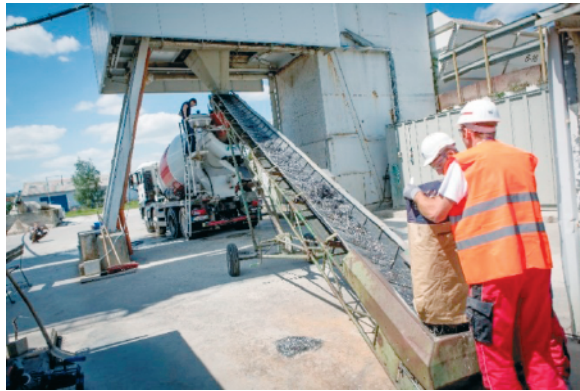
Figure 3. Fiber addition via conveyor belt (left) and filling of the beam from one side (right)
