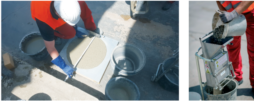
Figure 5. Determination of the flow spread (left) and separation of steel fibers from the fresh concrete (right)
