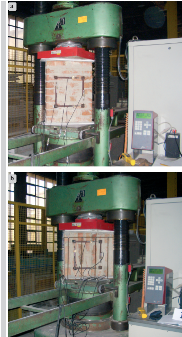
Figure 2. The masonry wallette type CV (a) and CH (b) with displacement measuring system – machine ready for testing
