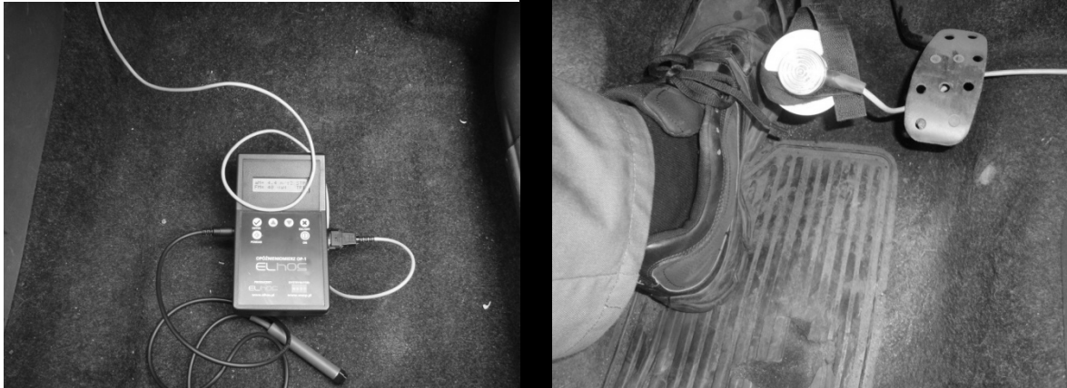
Fig. 6. OP-1 decelerometer and brake pedal pressure sensor used in the tests
