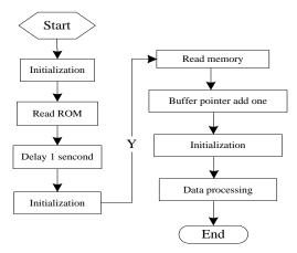
Figure 6. The flow chart of temperature collection
