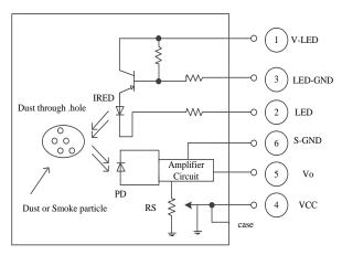
Figure 2. The structure of the dust concentration sensor
