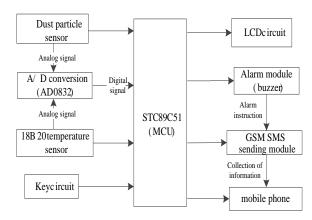
Figure 1. System structure diagram
