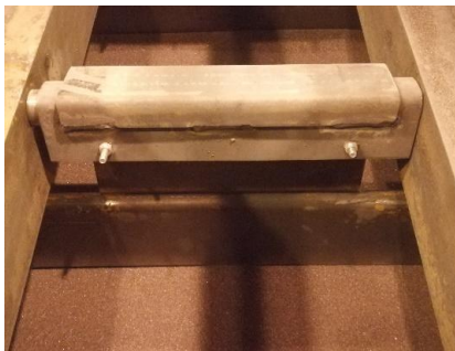
Figure 5. Physical map of trapezoidal scraper
