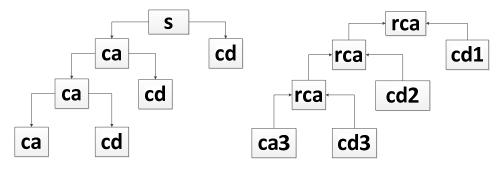
Figure 1. Wavelet decomposition tree and reconstruction tree
