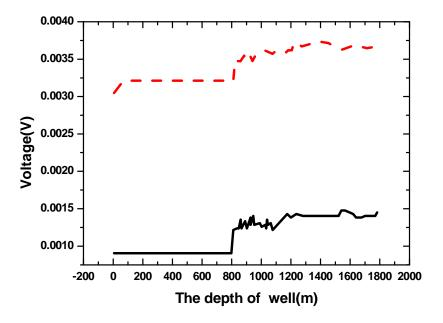
Figure 5. Stokes Raman and anti-Stokes Roman scattered signal
