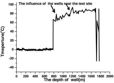
Figure 6. The original signal of well temperature test
