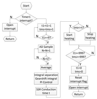
Figure 3. Timer 1 interrupt subroutine flow chart
