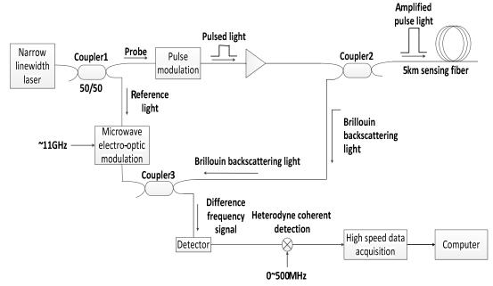
Figure 2. The basic structure of topic implementation plan
