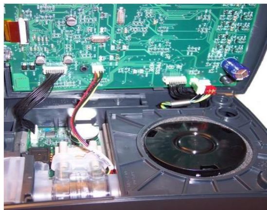
Figure 4. BLDC motor used in sleep-apnea equipment is able to remove a motor noise source.
