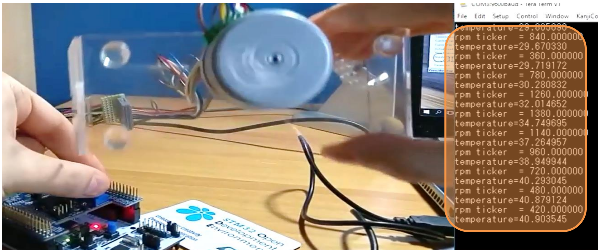
Figure 33. BLDC motor rotation with variable speed by changing on board potentiometer value; on the right, the variations of motor rpm value and temperature of L6230 IC driver.
