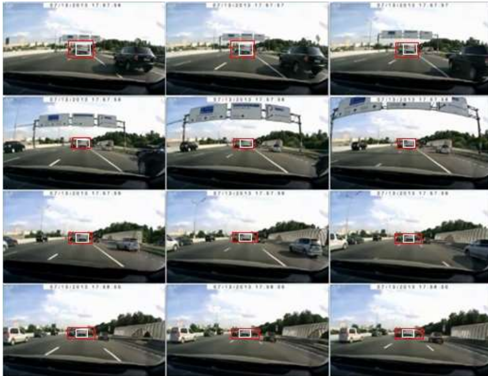
Figure 11. Detecting and tracking running truck in express way with dynamic noisy background caused by similar cars (white squares stand for N-SVDD, red squares stand for Mean-Shift)
