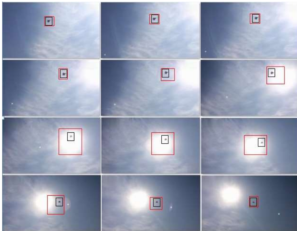
Figure 12. Detecting and tracking aircraft in clear sky with a high noisy background caused by strong sunlight (black squares stand for N-SVDD, red squares stand for Mean-Shift)
