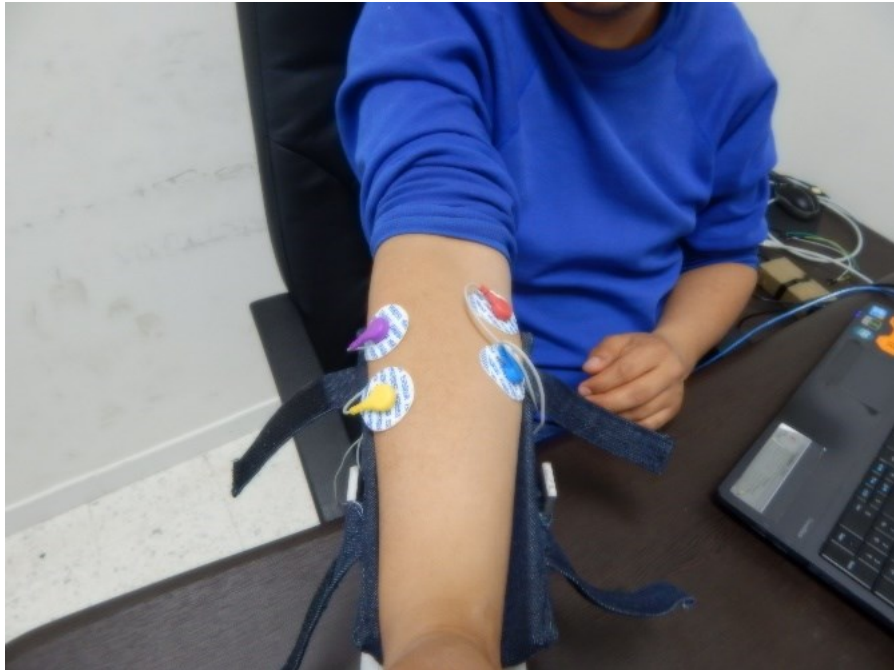
Figure 16. SEMG electrodes placed in the FCR and ECU muscles
